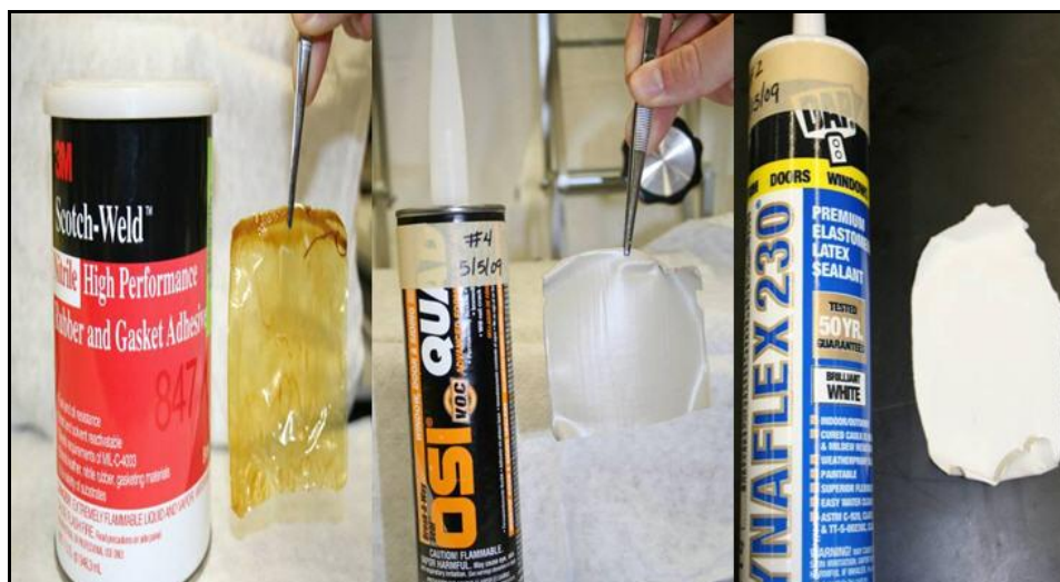
Figure 5. Dried films of 3M-847 (left), Quad (middle), and Dynaflex 230 (right).
