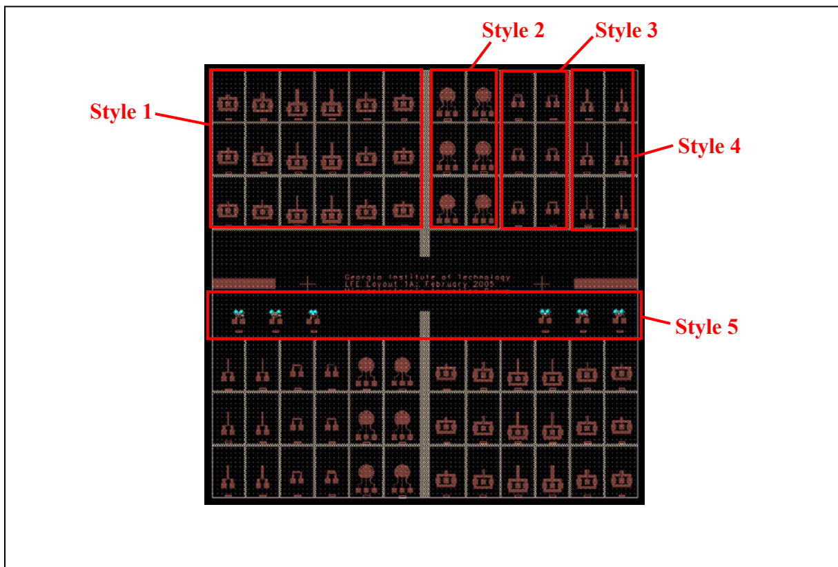
Figure 2. LFE I Die which includes 42 different electrode configurations that could be superimposed to form a 2-layer electrode configuration for more efficient LFE. Die measures 10 mm x 10 mm, arranged to fit 36 dice per photo-mask.
