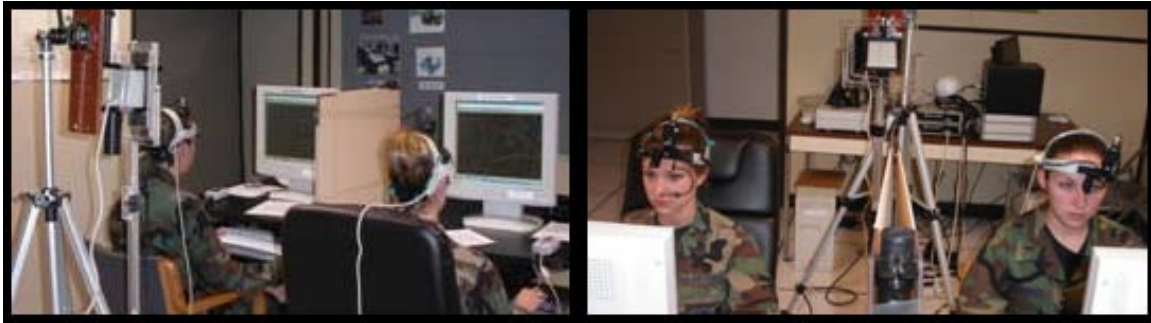
(A) (B) Figure 2. (A)Two ASL head- mounted eye trackers were used to record eye movements. (B) A divider prevented observers from viewing each others' screens.
