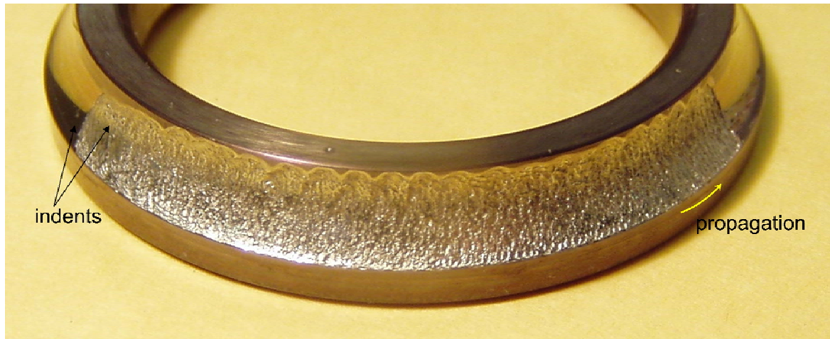
(a) Spalled M50NiL inner raceway
