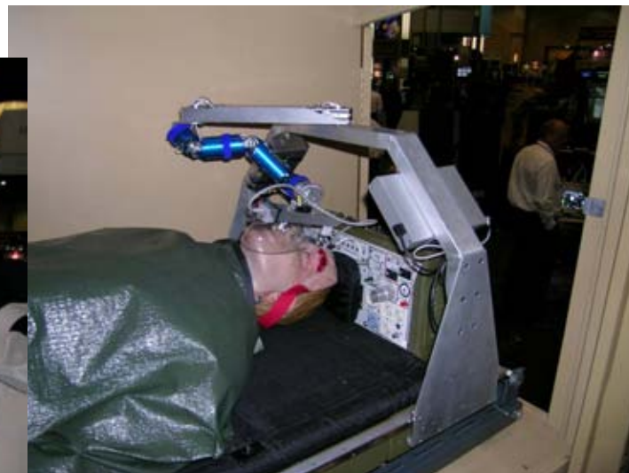
The robotic Serpentine Manipulator Arm and movable Gantry is housed in the TAGS UGV.
