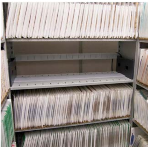
RFID labels were attached to paper medical records at Darnall AMC and outlying clinics. An unobtrusive shelf antenna system under the paper records enables rapid access through their RFID labels.
