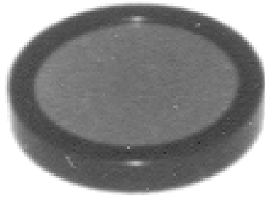
Fig. 8.15. Photograph of the recorded on-axis holographic parabolic mirror.
