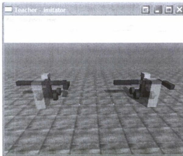
Fig. 1: Simulation setup with the two robots. The teacher robot is on the left and the learner on the right. The agents are performing the close left elbow action.
