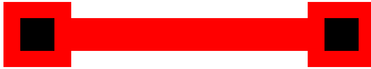
Figure 2.3: Sample dogbone resistor
