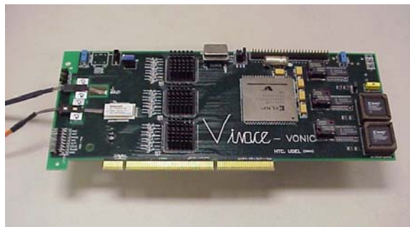
Figure 37. VIVACE Optical Network Interface Card (VONIC). Board dimensions are 25.7 cm x 10.7 cm x 157 mm.
