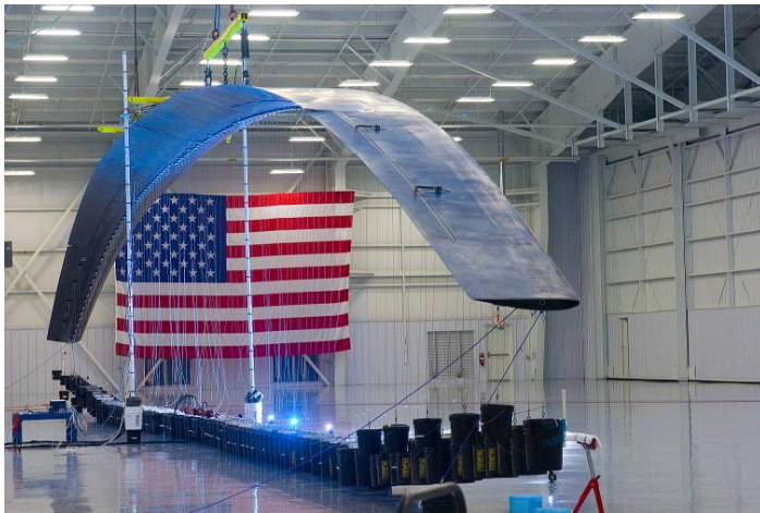
Wing in Design Limit Load test
