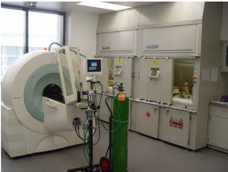
Figure 14: New radiochemistry facility at UT Southwestern: top left shielded hoods; top right hot cell; lower left PET/CT.
