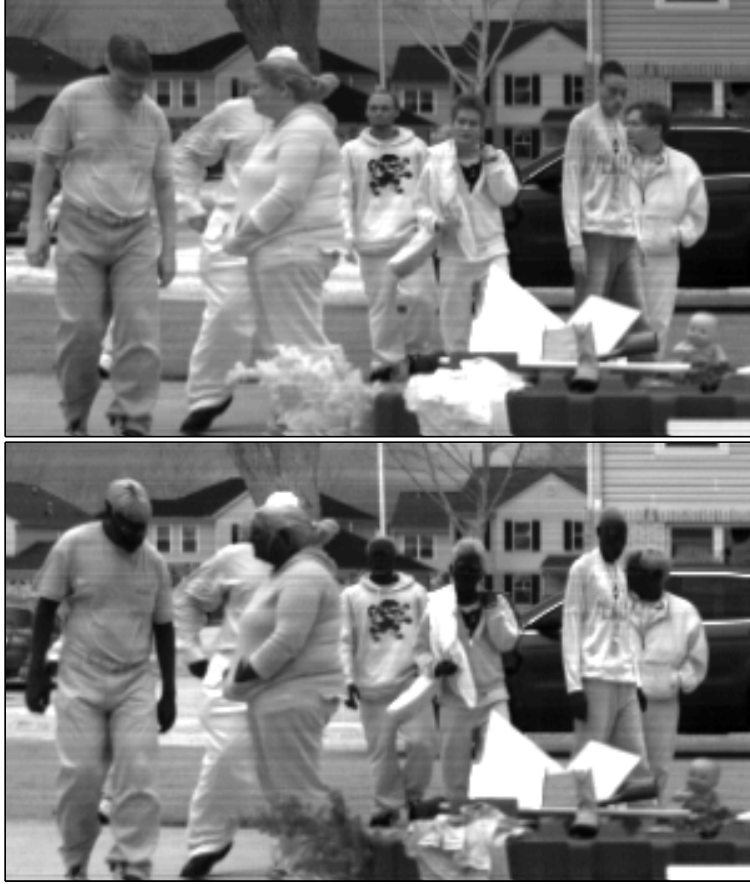
Figure 60: Suburban test scene with potential false alarm sources. Top: Image at 1080nm and Bottom: Image at 1580nm (bottom).
