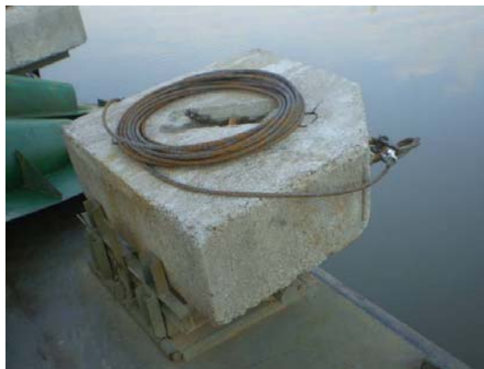
Figure B-2. Sinker and mooring on kickboard.
