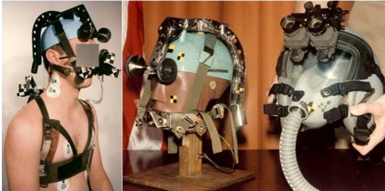
Figure 10: The added head mass apparatus used in the vertical accelerator experiments. The addition of weights replicates the masses of the helmet-mounted devices that aviators would likely be wearing in a dynamic event. Each volunteer's fiberglass helmet was custom fit to minimize relative movement.
