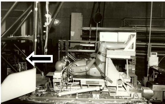
+Z: Runs were completed on both the horizontal accelerator (left) and vertical accelerator (right). +Z axial accelerations simulate aircraft ejection and ship shock.
