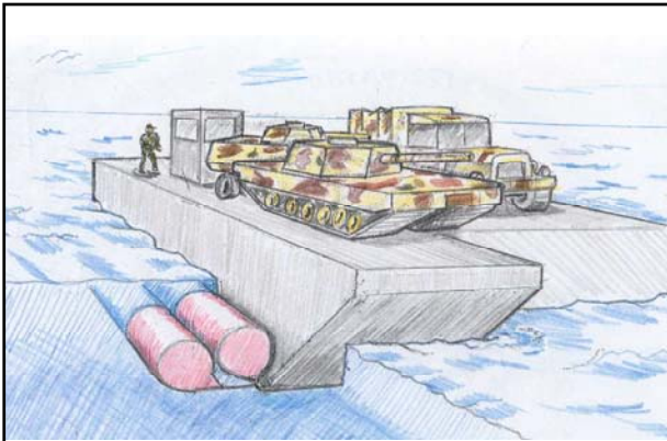
Concept F. Supplemental buoyancy to decrease CF draft (for marginal beach gradients).
