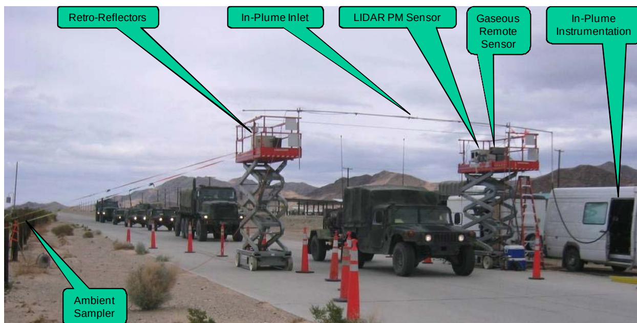
Figure 5-10. Picture of sampling system of In-Plume and Cross-Plume sampling.
