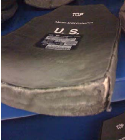
Figure 16. ESAPI at Fort Bragg With an External Material Failure
