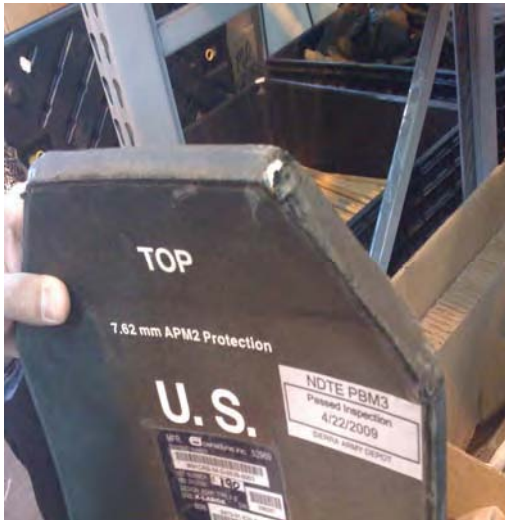
Figure 21. ESAPI at Fort Lewis with a Passed Inspection Label and an External Material Failure
