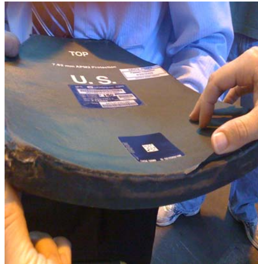
Figure 22. ESAPI at Fort Lewis with a Passed Inspection Label and an External Material Failure
