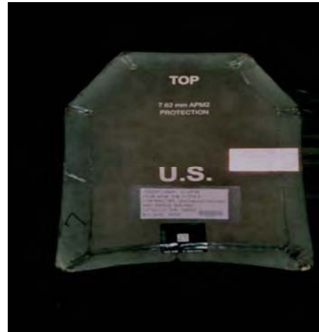
Figure 17. ESAPI at the IOTV Distribution Center With an External Material Failure and a Passed Inspection Label
