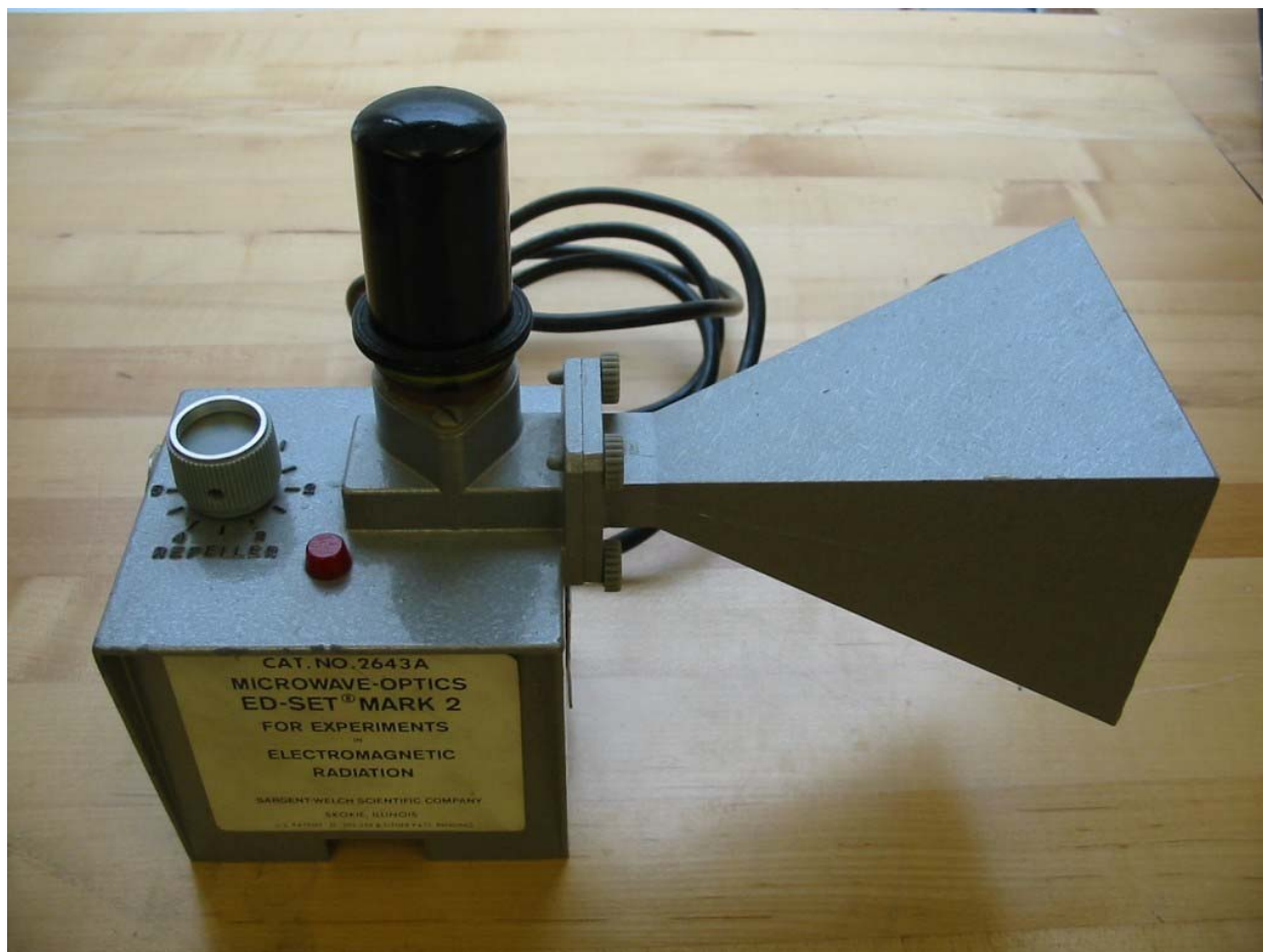
Figure 6 - 10.5GHz 15mW emitter acquired from the physics department.
