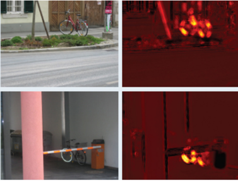
Fig. 5. Image classification via sparse modeling. Two classes have been considered, “bikes” and “background,” and the dictionaries were trained in a semi-supervised fashion [47].
