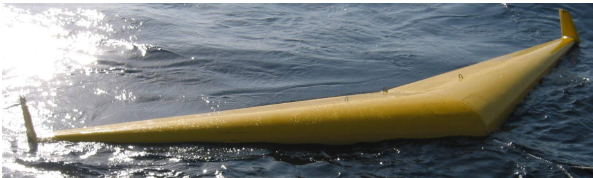
Figure 3. A prototype autonomous glider during initial sea trials. The “Liberdade” class of glider, developed with ONR support at the Scripps Institution of Oceanography, incorporated four Bioacoustic Probes to gather attitude and acoustic data during initial trials in April 2004.
