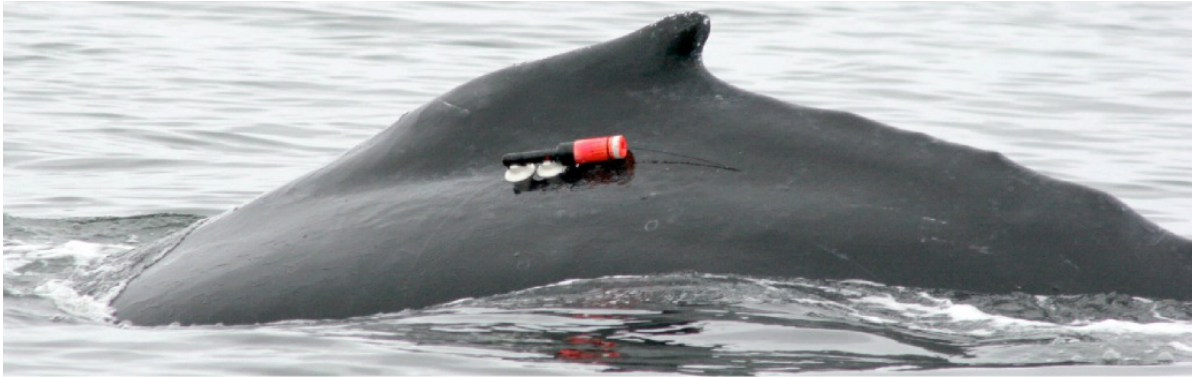
Figure 1. The Bioacoustic Probe attached to a humpback whale. Greeneridge Sciences' original acoustic recording tag, developed under contract to ONR during 1999–2003 and discontinued in 2007 (photograph courtesy John Calambokidis, Cascadia Research).
