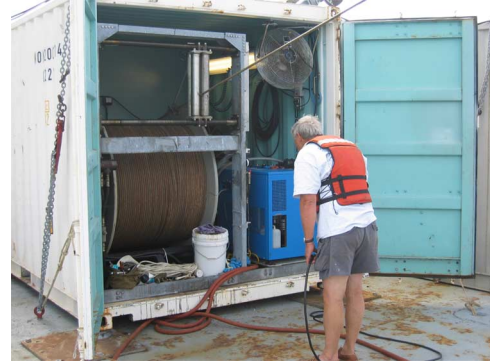
Fig. 3. Source deployment winch with 1.7-cm cable (standard 0.68-in oceanographic cable), and one of two air compressors, all mounted in one half of a 20-ft van. The other half of the van housed the power amplifier, signal generation electronics, and a computer.
