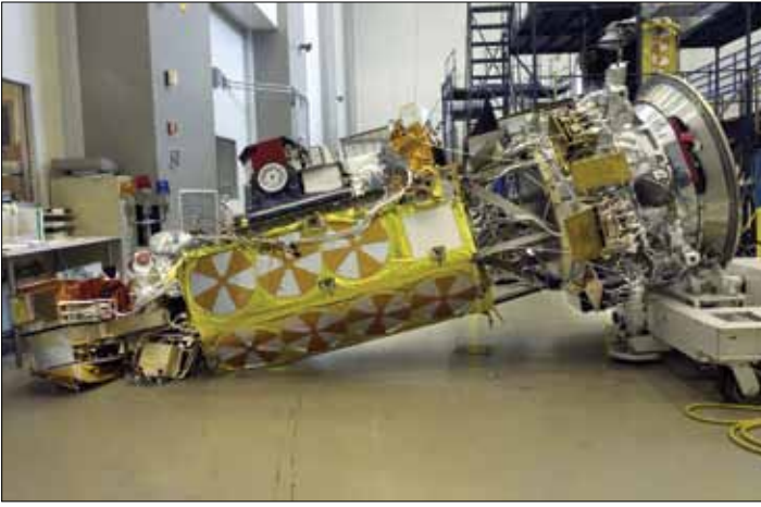
While performing work on the NOAA-N Prime spacecraft, being prepared to launch in 2008 for the National Oceanic and Atmospheric Administration (NOAA), the satellite was dropped.
