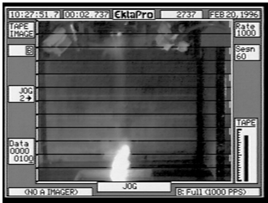
Sphere Discharge (2 ms after Detection) (Water 35 inches above Tabletop)
