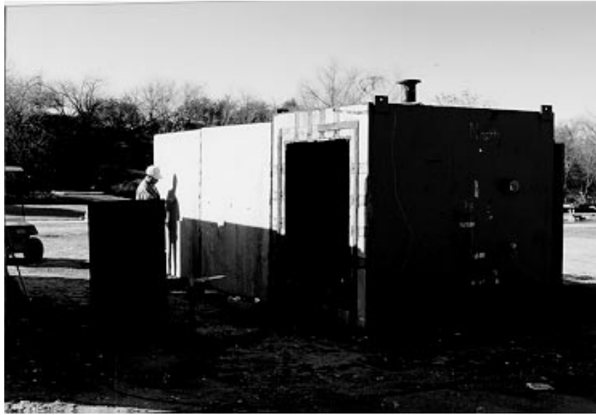
Figure 2.4 Photo of Large Test Chamber and Concrete Reflecting Walls Parallel to Front Opening
