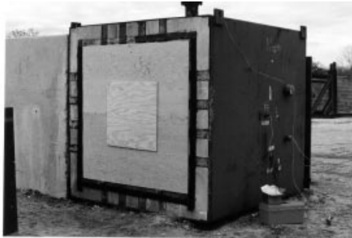
Figure 2.2 Photo of Large Blast Chamber Showing Attached Vent Panel
