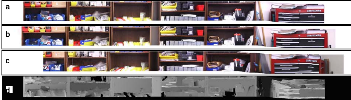
Fig. 14. Multi-view stereo mosaics for an indoor scene. (a) The leftmost, (b) center and (c) the rightmost views of total eleven mosaics. (d) the height map generated.
