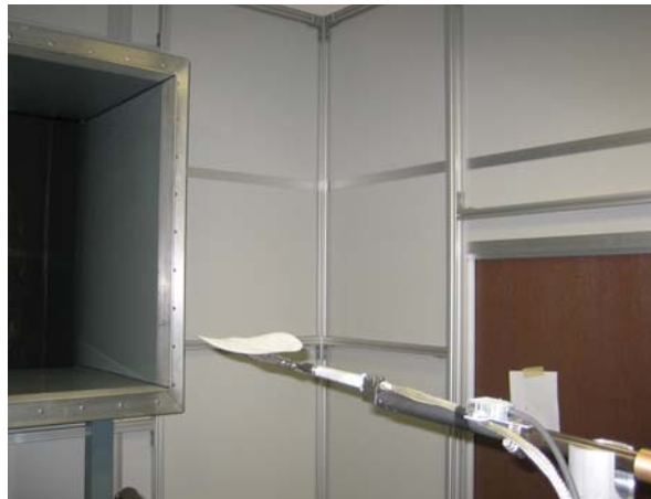
Figure 2. The MAV wing in the wind tunnel. The model is attached to the two D.O.F. rig through the sting balance.
