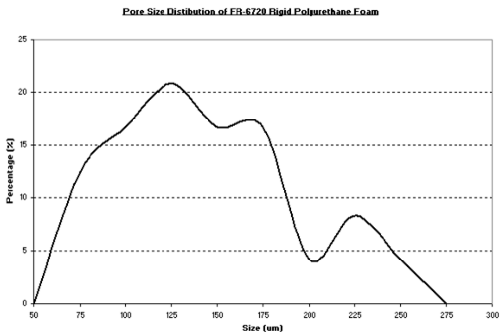
Figure 27. Pore Size Distribution of FR-6720 Polyurethane Foam
