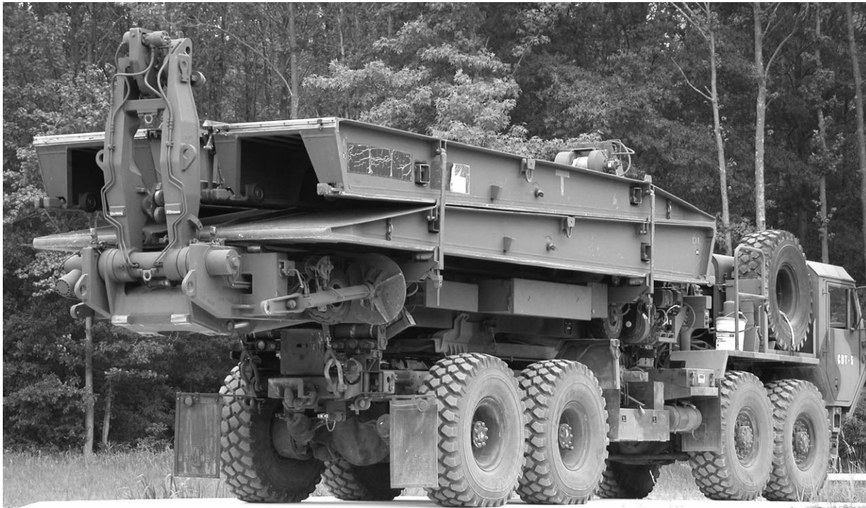
Figure 7. Army bridging system
