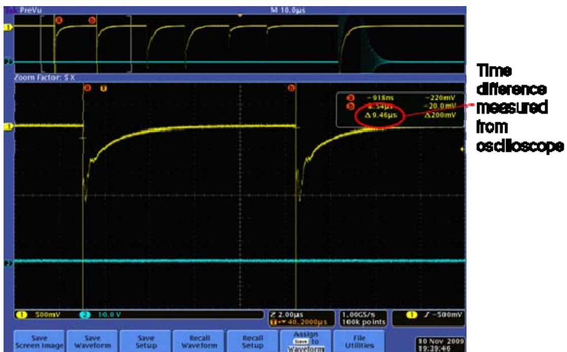
Figure 42. Time Difference Measured on Oscilloscope
