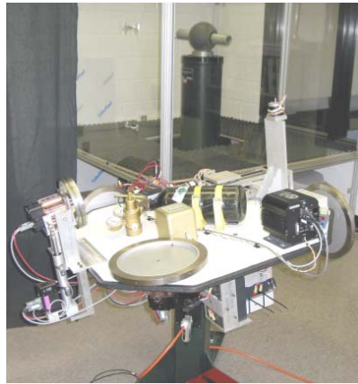
Figure 10. Virginia Tech Distributed Spacecraft Attitude Control System Simulator (DSACSS) (Whorl I, left; Whorl II, right) [From 27]
