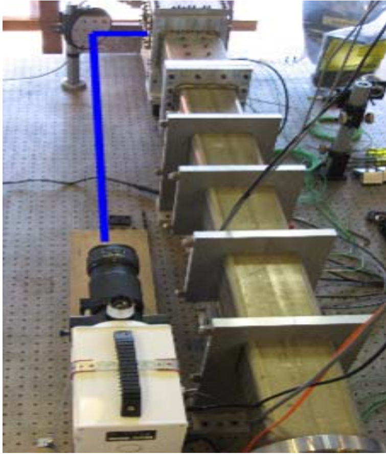
Figure 25. Photo and Diagram Illustrating Camera Setup for Flame Imagery.
