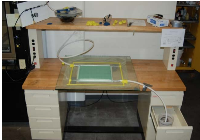
Figure 1. Fabrication of samples by VARTM process
