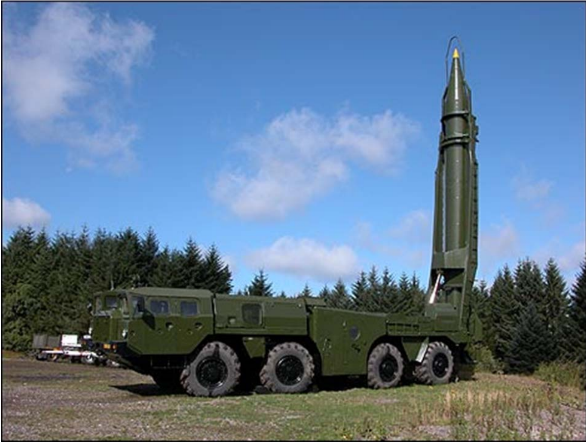
Figure 16. SCUD Transporter Erector and Launcher (TEL) 102
