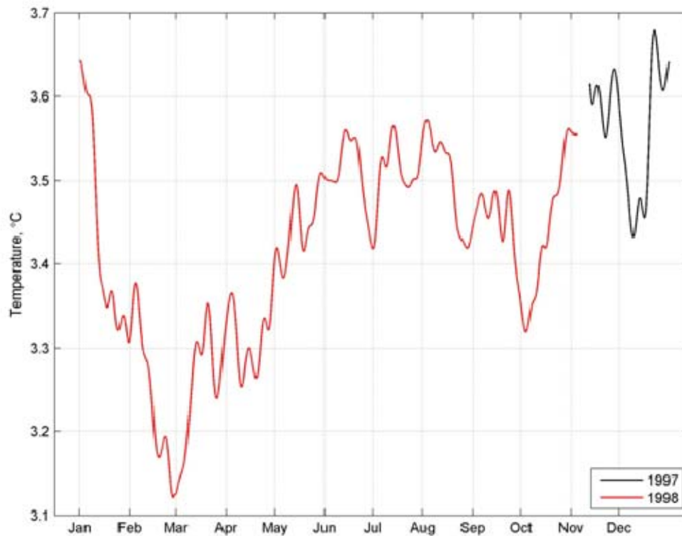
Figure C9. Temperature time series of currents at mooring D2. Temperatures were smoothed using a Butterworth filter that cut off periods less than one week.
