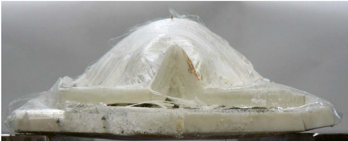
Figure 54. Cross Sectional View of the Actual Composite Plate (C-D1) for Comparison.
