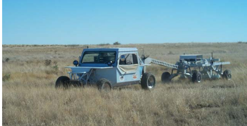
Figure 5-2 – MTADS tow vehicle and magnetometer array.
