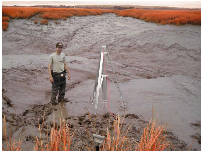
Figure 2. The K-probe ( K_{1C} ) deployed in a muddy tidal flat sediment. (PhD student Mark Barry for scale.)
