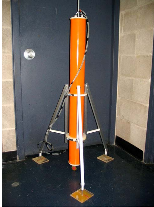
Figure 3. The improved E-probe standing in the lab at Dalhousie. The expandable bladder, which is at the heart of the probe, is observable as the red “dot” at the base of the instrument tube.
