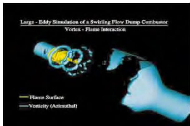
Figure 3. Large-eddy simulation of a swirling flow in a combustor showing the vortex flame interaction
