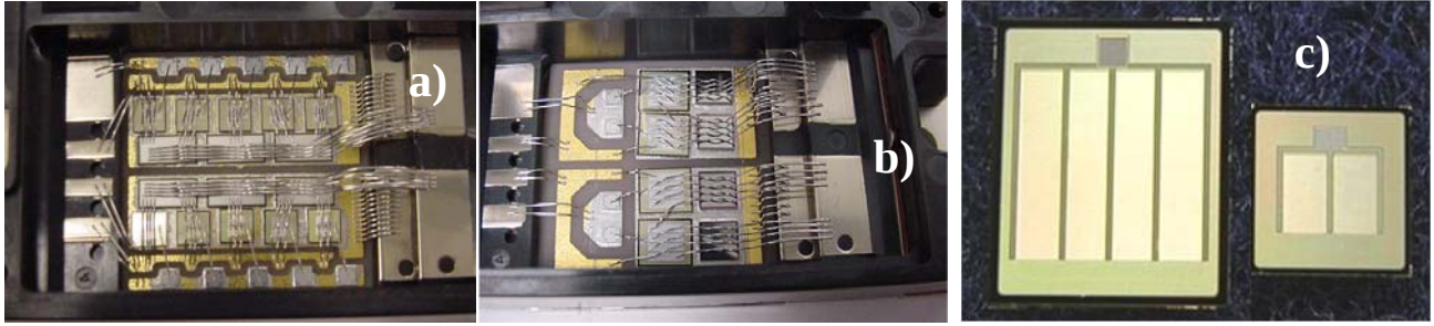
Figure 1. SiC module die layout for a) 20 A MOSFETs, b) 80 A MOSFETs, and c) die.
