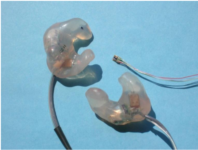
Figure 4. Indy Racing League type earplugs made by Sensaphonics (three Delphi AD 193 linear sensors)
