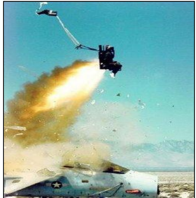
Figure 1 - Ejection Seat Testing Performed by the USAF
