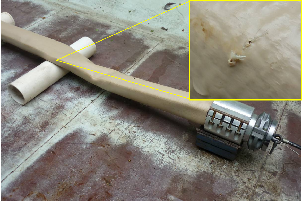
Figure 3.7 – Hose Sample D Failure
