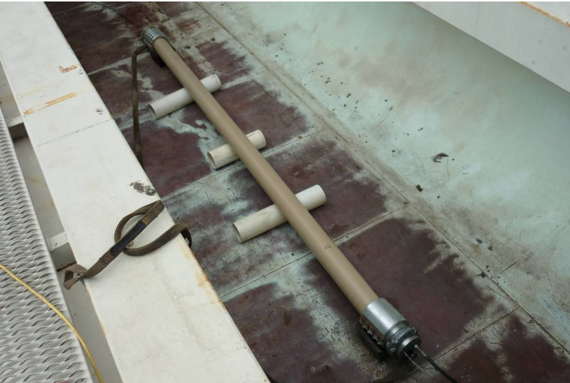
Figure 3.6 – Hose Sample D Burst Test Setup
