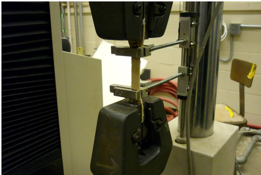
Figure 6.3 – Test Sample Mounted in Tensile Test Frame
