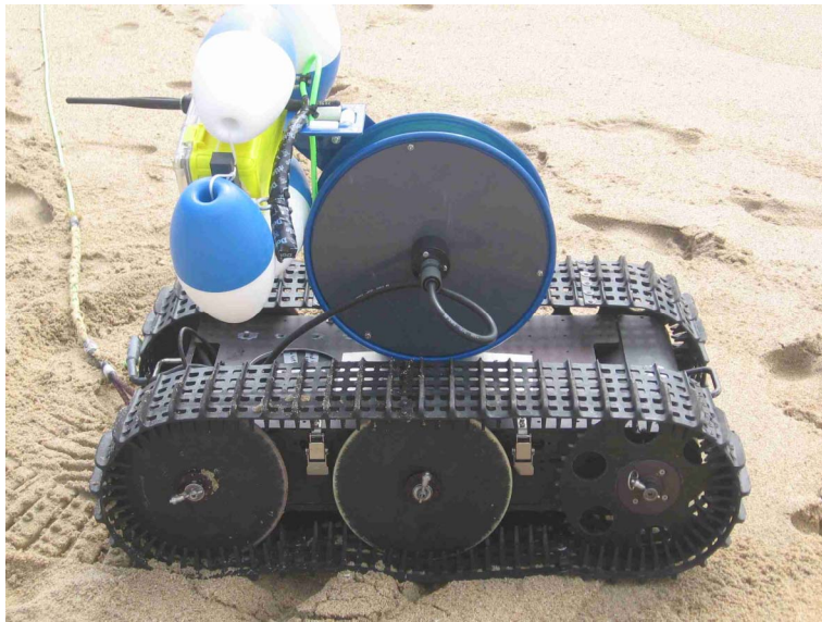
Figure 4. A crawler on a sandy beach before surf zone operation. A retractable reel and float (underwater box with GPS and radio communication, and positive buoyancy required for floatation) mounted on the platform.
