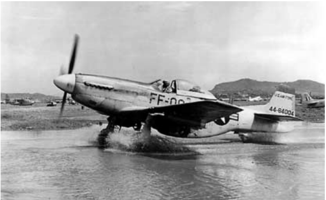
An F-51, loaded with one bomb on each inboard station and unguided rockets on its outboard stations, taxis through flooded conditions to take off at a Korean airfield.
