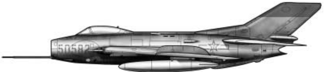
"The F-6 (Jianji-6 Fighter aircraft 6) is the Chinese version of the MiG-19, which as of the mid-1990s was still in production in China. The J-6, which began flight tests in 1958, was China's first supersonic jet fighter." (From "MiG-19 Farmer, J-6/F-6," Federation of American Scientists, 26 June 2000, on-line, Internet, 2 June 2003, available from http://www.fas.org/nuke/guide/russia/airdef/mig-19.htm .)
