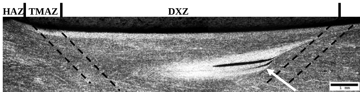
Figure 2. Typical FSP zone, shown from section processed at 800 RPM and 50 mm/min.
