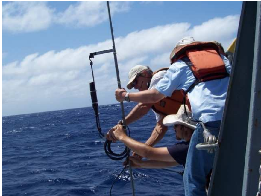
Figure 63: Attaching the monitor hydrophone and its bungy mounting frame to the suspension cable over the stern of the R/V Melville during deployment.
