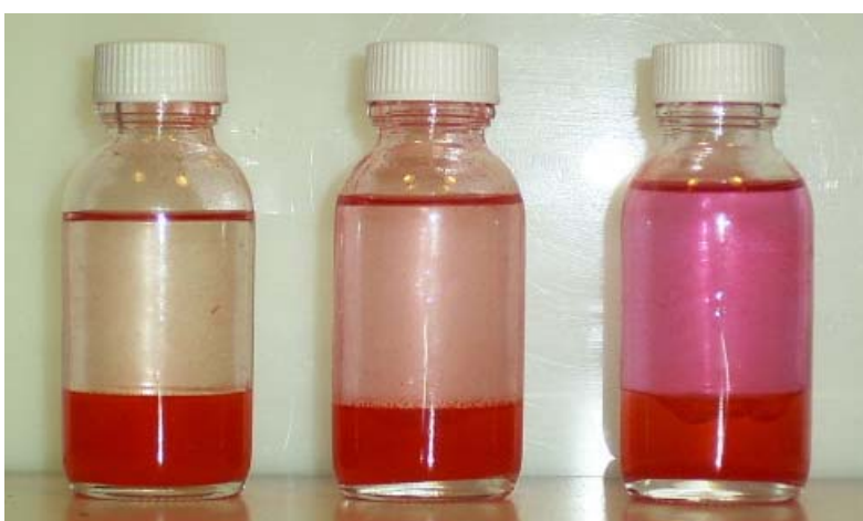
Figure 2: Erythrosine red dye dispersant test for +100 in jet fuel Samples from left to right are 0 ppm, 100 ppm and 256 ppm of S-1749 additive. A colour change of the top phase indicates the presence of the additive.
