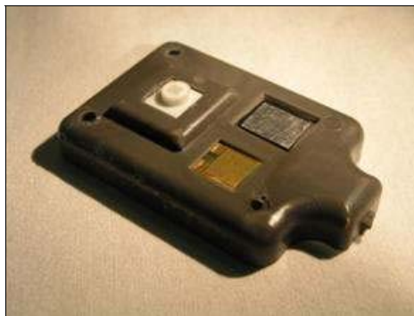
Figure 1: Corrosion, wetness, temperature and humidity sensors packaged with the interface and networking electronics into one small, low-power and light unit. This has been developed under a collaborative project with MiniFAB (Aust) Pty. Ltd., an SME based at Scoresby, Melbourne.
