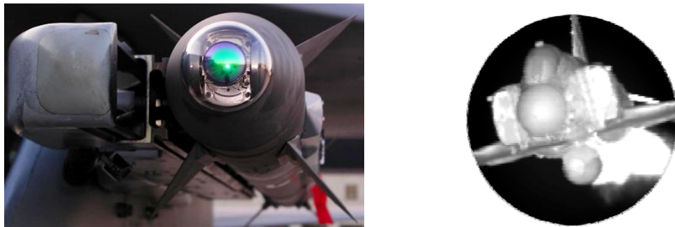
Figure 2: AIM-9X Seeker head and digital imaging (Jane's Defence Online)
