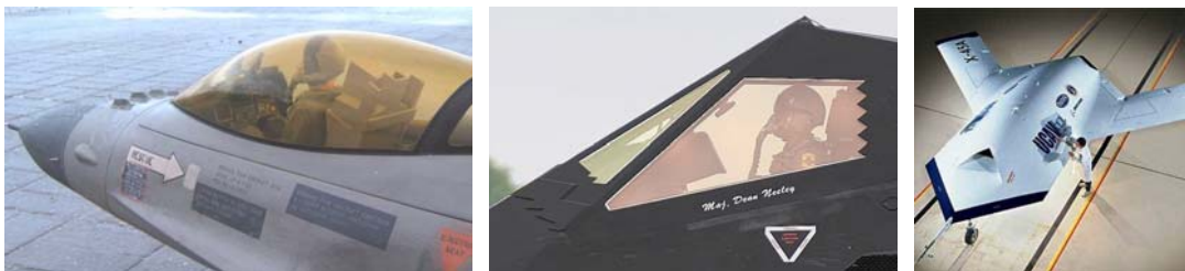
Figure 8: Efforts to reduce RCS: gold canopy, saw-tooth edges, raised engine nacelle
