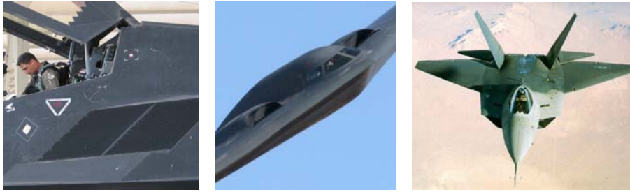
Figure 7: Efforts to reduce radar cross-section; mesh screens, raised nacelles, canted tails
